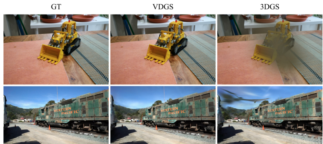
Figure 18. Comparison results between VDGS [36] and original 3DGS [6] on Tanks and Temples [59] and Mip-NeRF 360 [58] datasets. Note that VDGS renders fewer artifacts in both datasets compared to original 3DGS. Figures come from [36].
